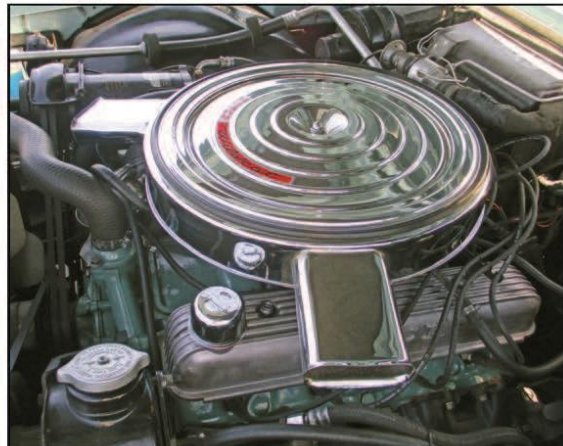
Dual-quad Super Wildcat engine with the chrome air cleaner and ribbed aluminum valve covers.
